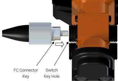
! Make sure key is inserted and connector is fully screwed in. Fiber optic signal losses will significantly increase if not connected properly.
