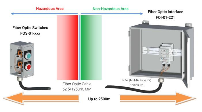
The system provides a safe optical signal (rated inherently safe **Ex op is**), which can be used in any type of hazardous environment or explosive atmosphere.
