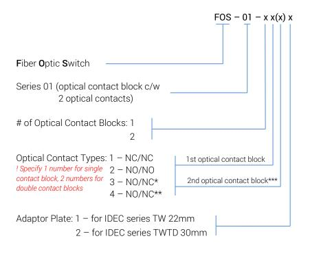
\* "Break-Before-Make" contacts. NC contact opens before NO contact closes.
